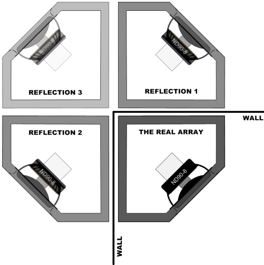
Figure 2-11: Top View of the Single Corner-Line-Array with Three Reflections
