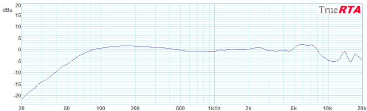
Figure 4-6: ND90 Nearfield/Ground Plane Hybrid Closed Box Response (0.1 cubic foot)
