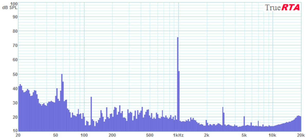
Figure 4-10: The ND90 at 1000 Hz, 1Watt, 1 meter
