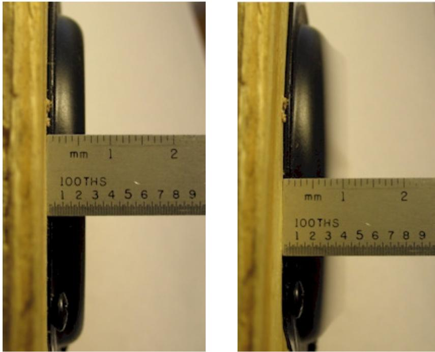
Figure 4-3: The ND90-8: excursion baseline (left) and 50 Hz at 10% 3rd harmonic distortion. (right)
