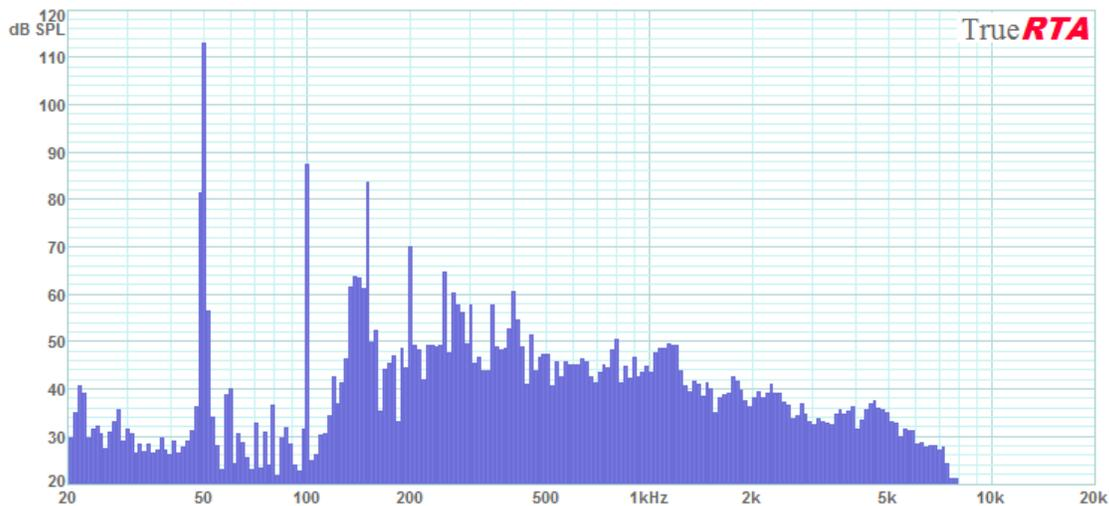
Figure 5-13: The Array's Sine Wave Spectrum at 50 Hz for 65 Watts Input at 1 meter
