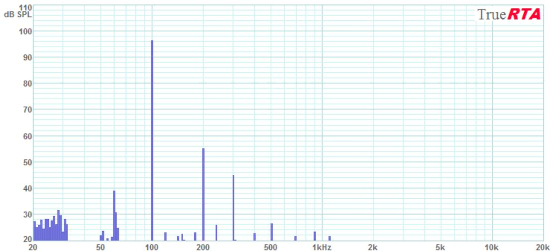
Figure 5-8: The Array's Sine Wave Spectrum at 100 Hz for 1 Watt at 1 meter
