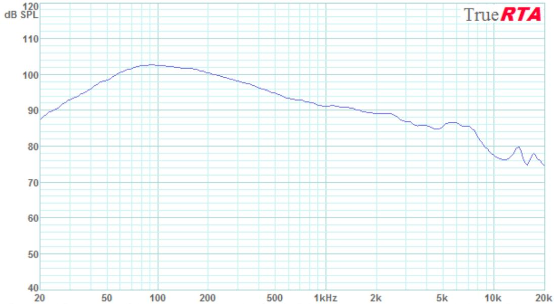
Figure 5-5: Predicted Response of the Array based on the Single Driver Response summed with the -3 dB/octave Reference
