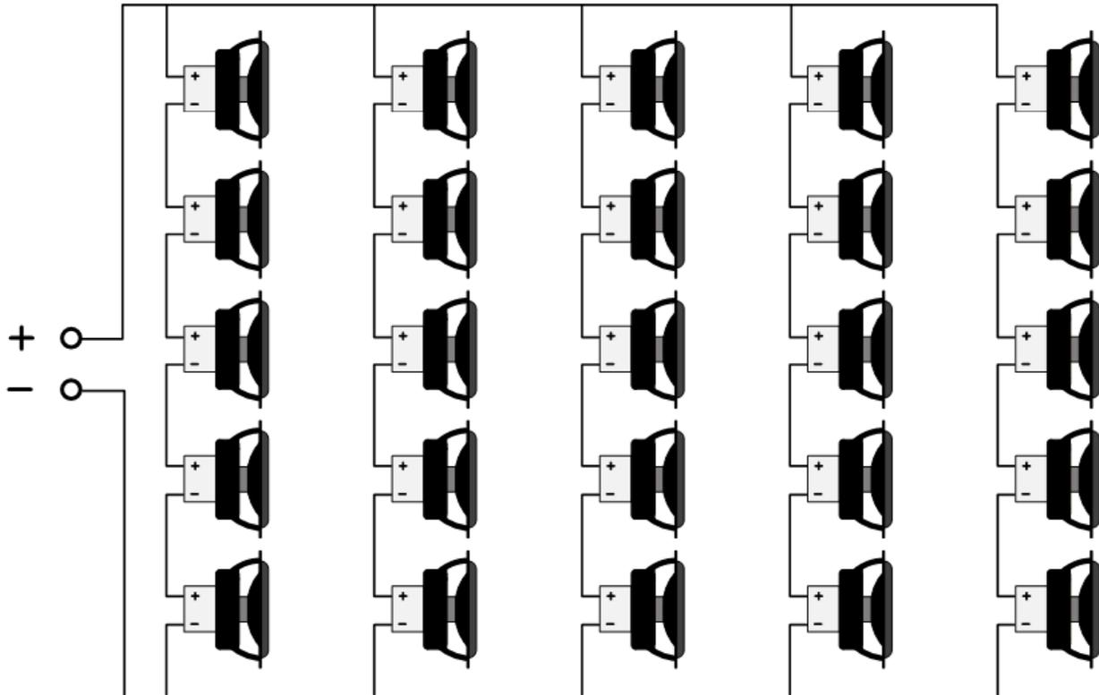
Figure 3-2: The MCLA Wiring Diagram for 25 Drivers
