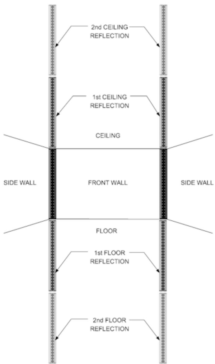
Figure 2-10: Line Arrays with Ceiling and Floor Reflections
