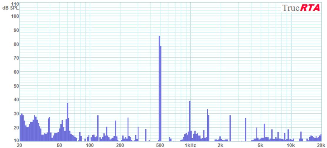
Figure 5-10: The Array's Sine Wave Spectrum at 500 Hz for 1 Watt at 1 meter
