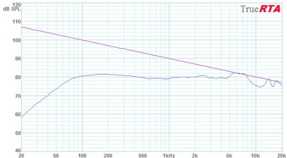
Figure 5-4: The Single Driver Half-Space Response along with a -3 dB/octave Reference
