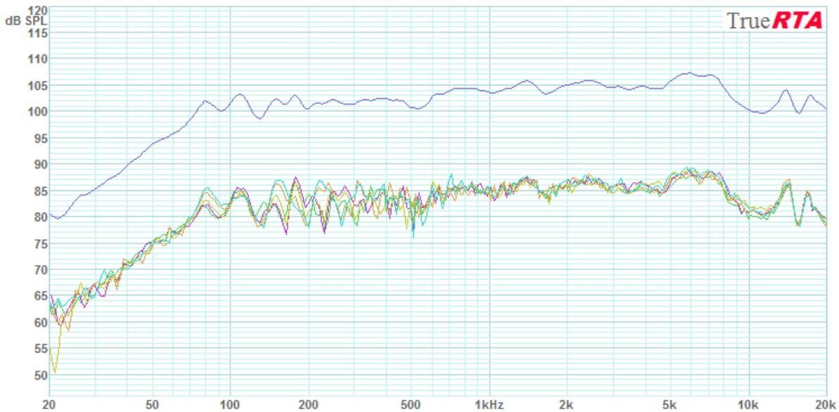
Figure 4-5: ND90 Ground Plane Frequency Response, Closed Box (0.1 cu ft), 1W/1m
