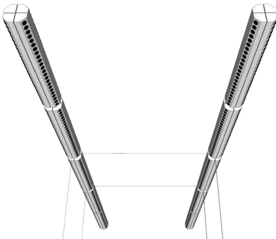
Figure 2-15: The In-Room Acoustic Equivalent of Just Two Murphy Corner-Line-Array Enclosures
