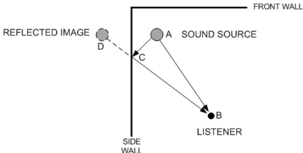
Figure 2-7: Sound Source with a Single Reflected Image
