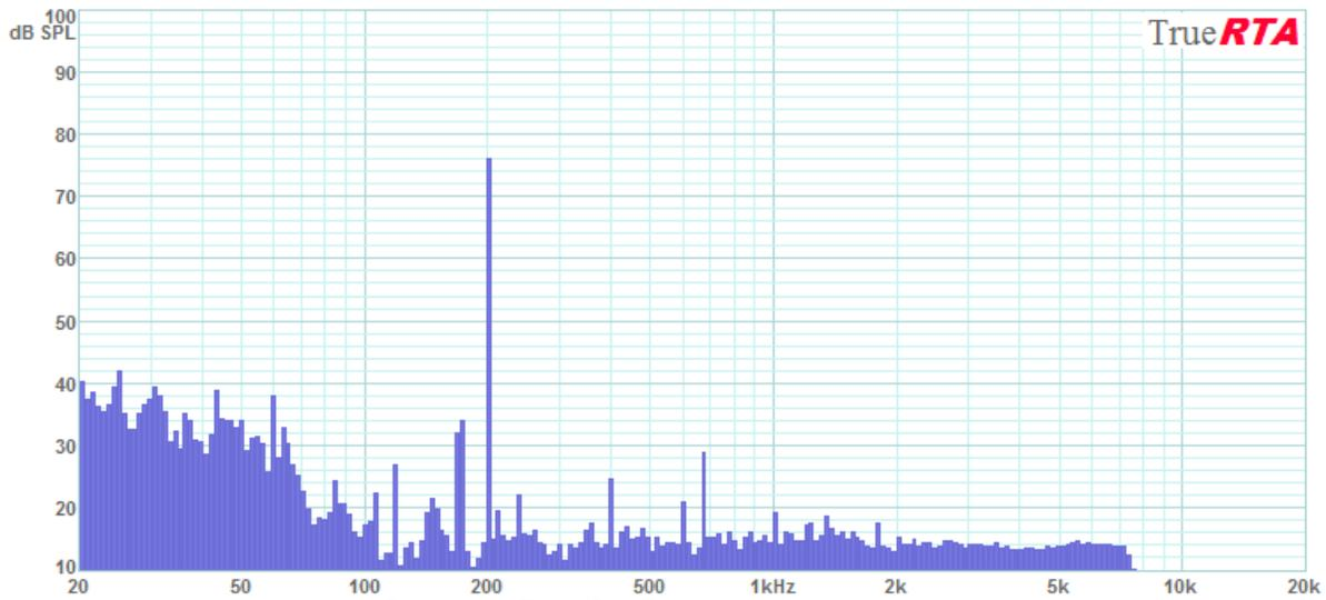
Figure 4-8: The ND90 at 200 Hz, 1Watt, 1 meter
