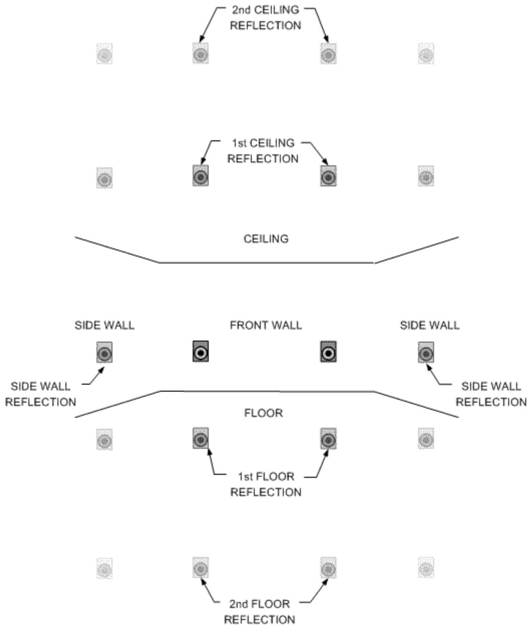
Figure 2-9: A Stereo Pair of Point Source Speakers and Their First Few Reflections
