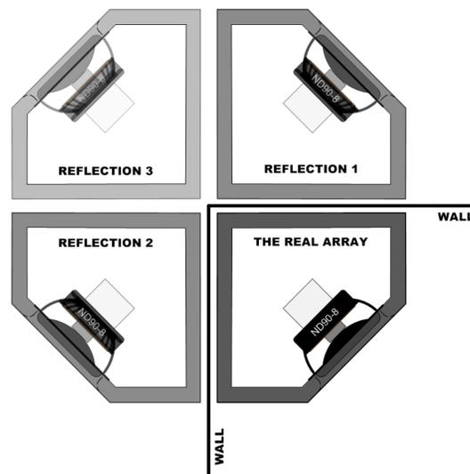
Figure A2-1: A Single Murphy Corner-Line-Array As Viewed From Above Along With Three Reflections
