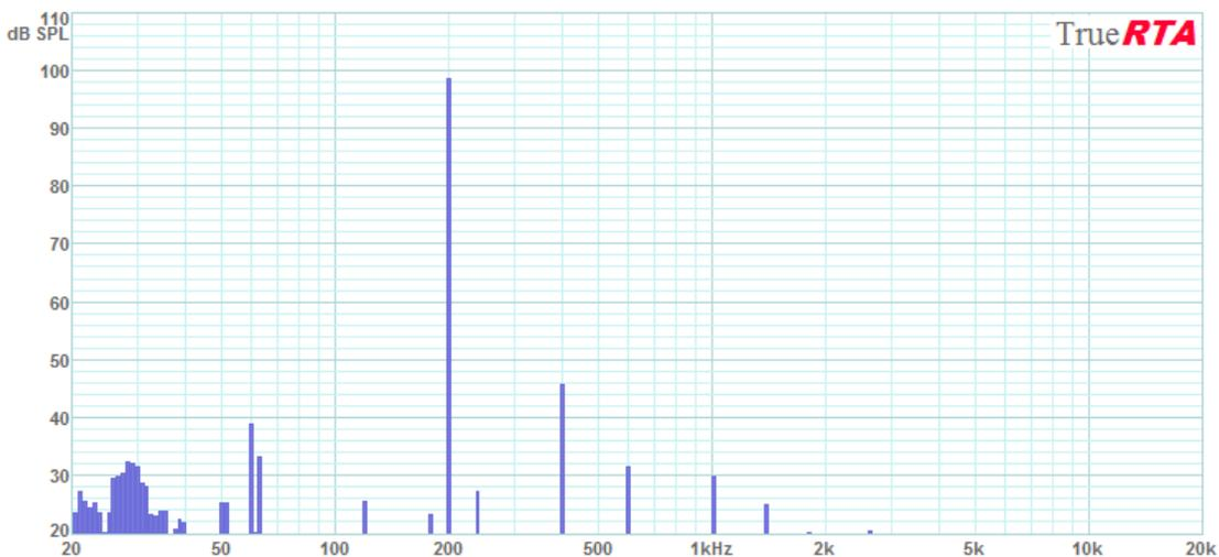
Figure 5-9: The Array's Sine Wave Spectrum at 200 Hz for 1 Watt at 1 meter
