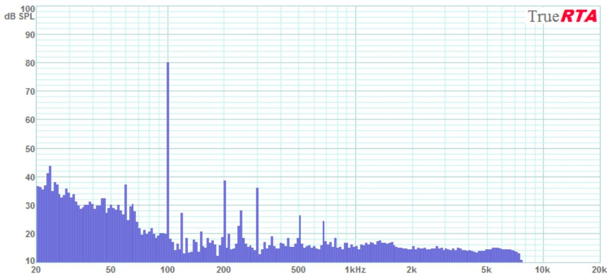
Figure 4-7: The ND90 at 100 Hz, 1Watt, 1 meter
