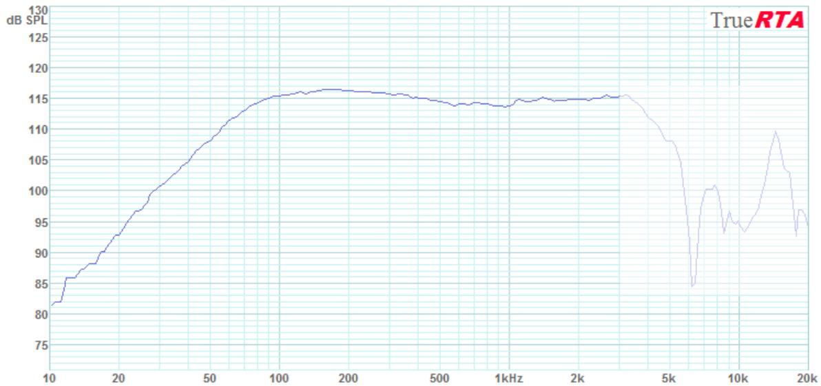
Figure 4-4: ND90-8 Nearfield Frequency Response in 0.1 cubic foot closed box (ignore above 3kHz)
