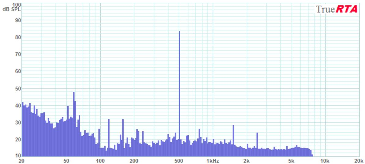
Figure 4-9: The ND90 at 500 Hz, 1Watt, 1 meter
