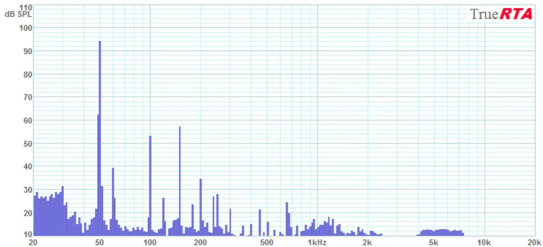
Figure 5-12: The Array's Sine Wave Spectrum at 50 Hz for 1 Watt at 1 meter
