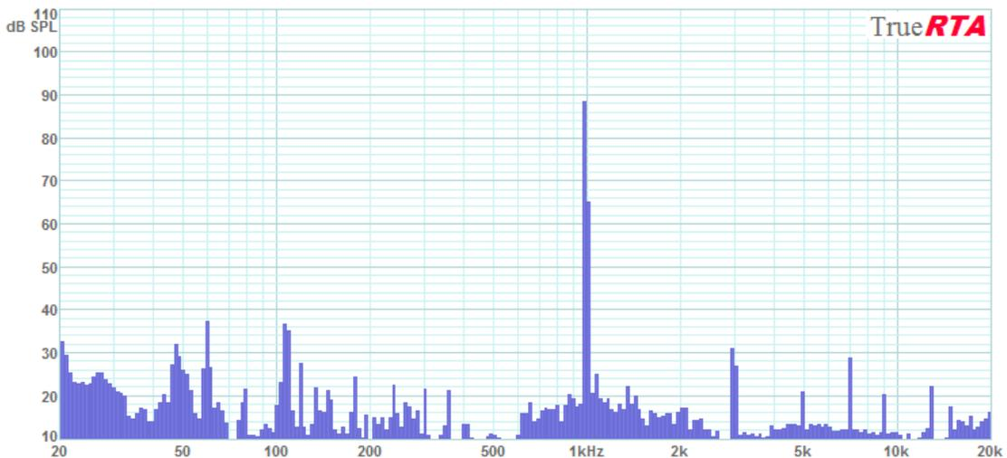
Figure 5-11: The Array's Sine Wave Spectrum at 1000 Hz for 1 Watt at 1 meter
