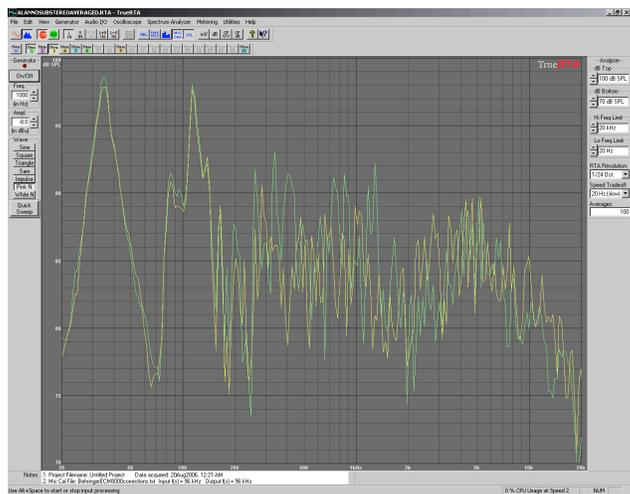
The second figure shows two graphs; the original frequency plot, plus another taken one foot to the left of the original measurement position. I have increased the scale of the graph so that similarities and differences between the two listening positions are more easily seen. Notice that the broad peaks in dips are nearly identical between the two listening positions up to about two hundred Hz, but then start to differ dramatically.
