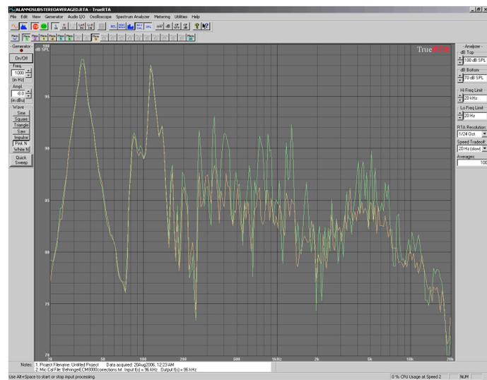
True RTA has features that enable you to average a number of measurements together. The figure below shows the prime listening position in green, and all listening position measurements averaged together in brown. The averaged measurements show the “BBC dip” that the designer of my speaker was nice enough to implement into the crossover. The average also shows the natural progressive attenuation of high frequencies that occur in a listening room.
