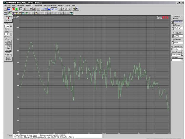
taken at the prime listening position in my listening room using the quick sweep measurement functionality of True RTA. The Y axis of the graph represents sound pressure level in decibels. The X axis represents the frequency range from 20Hz to 20kHz. Notice the average level falls at about 85dB with broad peaks and dips throughout the frequency range.
